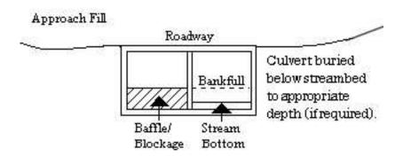
(7) Where adjacent floodplain is available, flows exceeding bankfull will be accommodated by installing culverts/pipes at the floodplain elevation. When multiple culverts/pipes are used, baseflow must be maintained at the appropriate width and depth by the construction of floodplain benches, sills, and/or construction methods to ensure that the overflow culvert(s)/pipe(s) is elevated above the baseflow culvert(s)/pipe(s).
